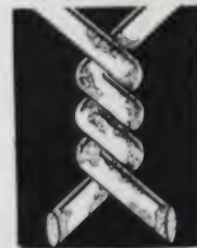
Observe how bending of pre-coated wire during weaving process causes zinc coating to crack and scale.
